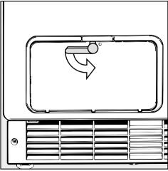
■ Turn the inner cover lock downwards to the vertical position.
